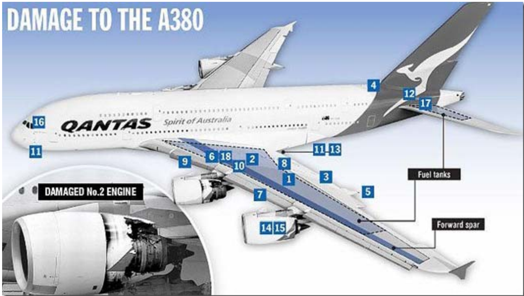
Qantas Flight 32, November, 2010 out of Singapore oil from bearing box leaked and ignited
